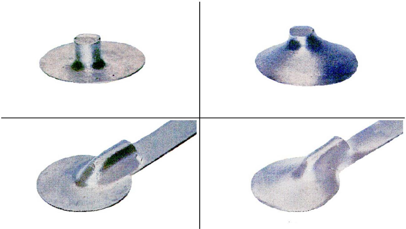
**Pictures of through-hole terminations showing minimum and maximum solder.**
