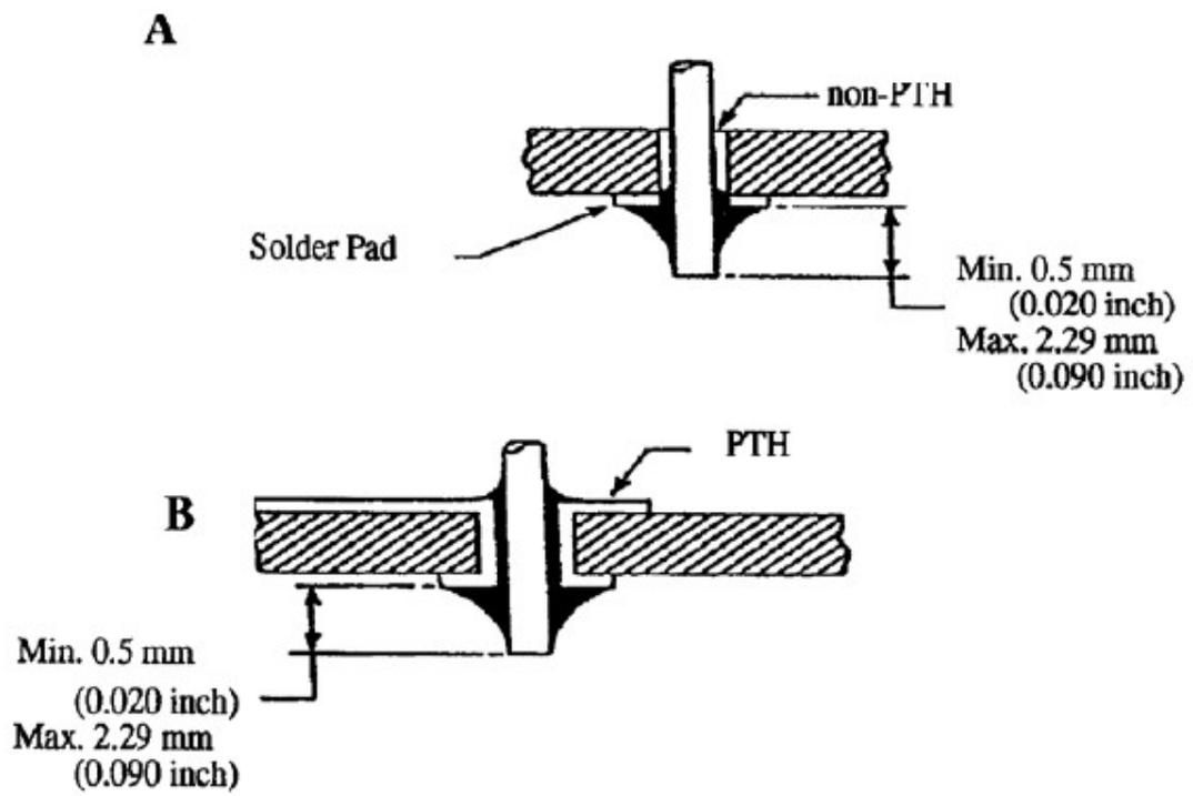
Figure 8-18. Straight-Through Termination
